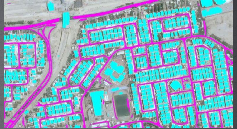
The algorithm recognizes both roads and buildings.
