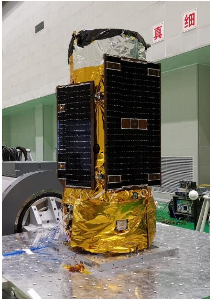
Jilin-1 GF04A satellite under the vibration test
