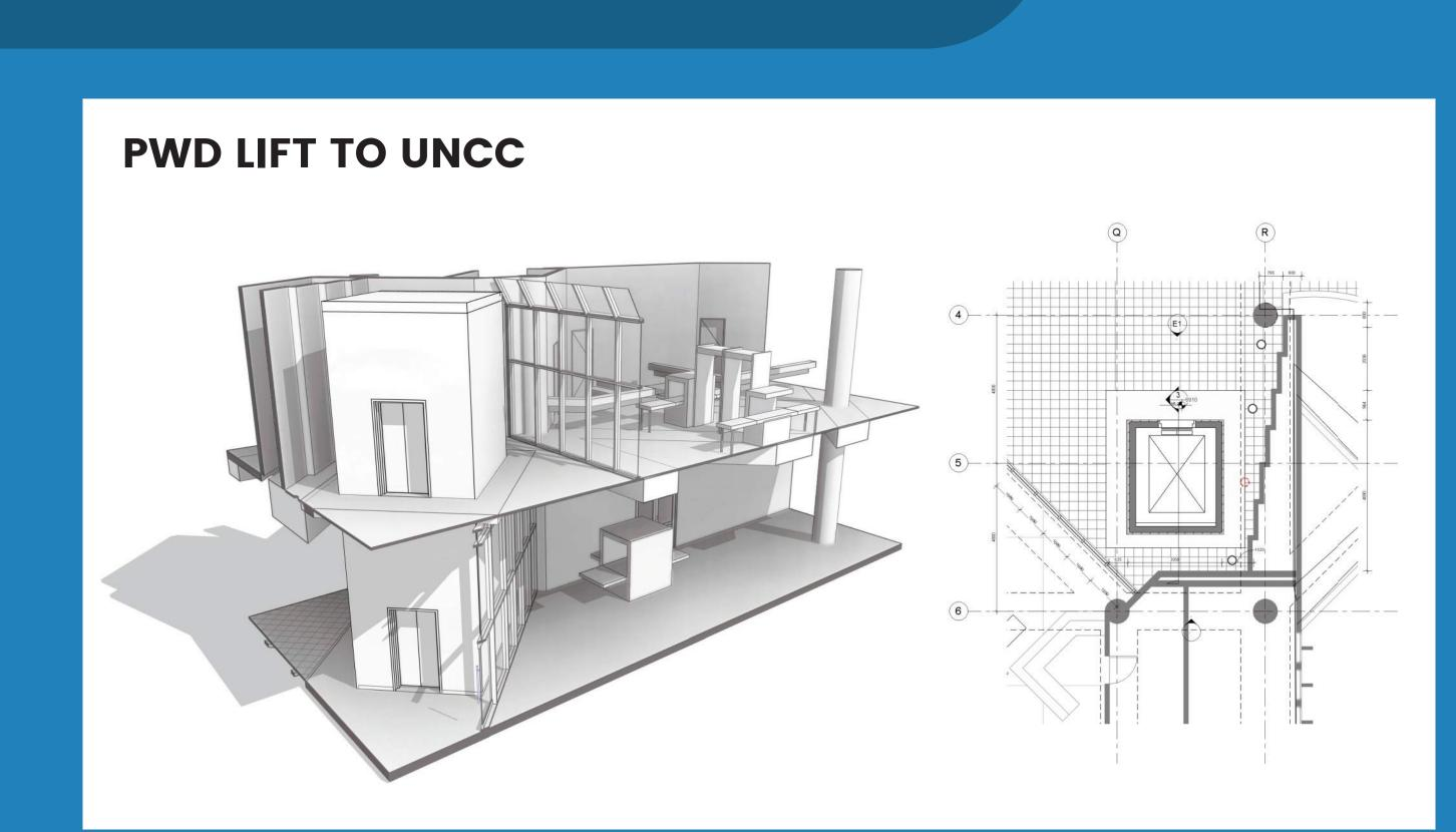
A proposed project is to provide a new stretcher/PWD compliant lift that provides a 9m vertical movement between the UNCC lower level, Ground level and Level 1. The lift's placement is external to the building, enabling the existing building's perimeter security strategy to remain unchanged.
