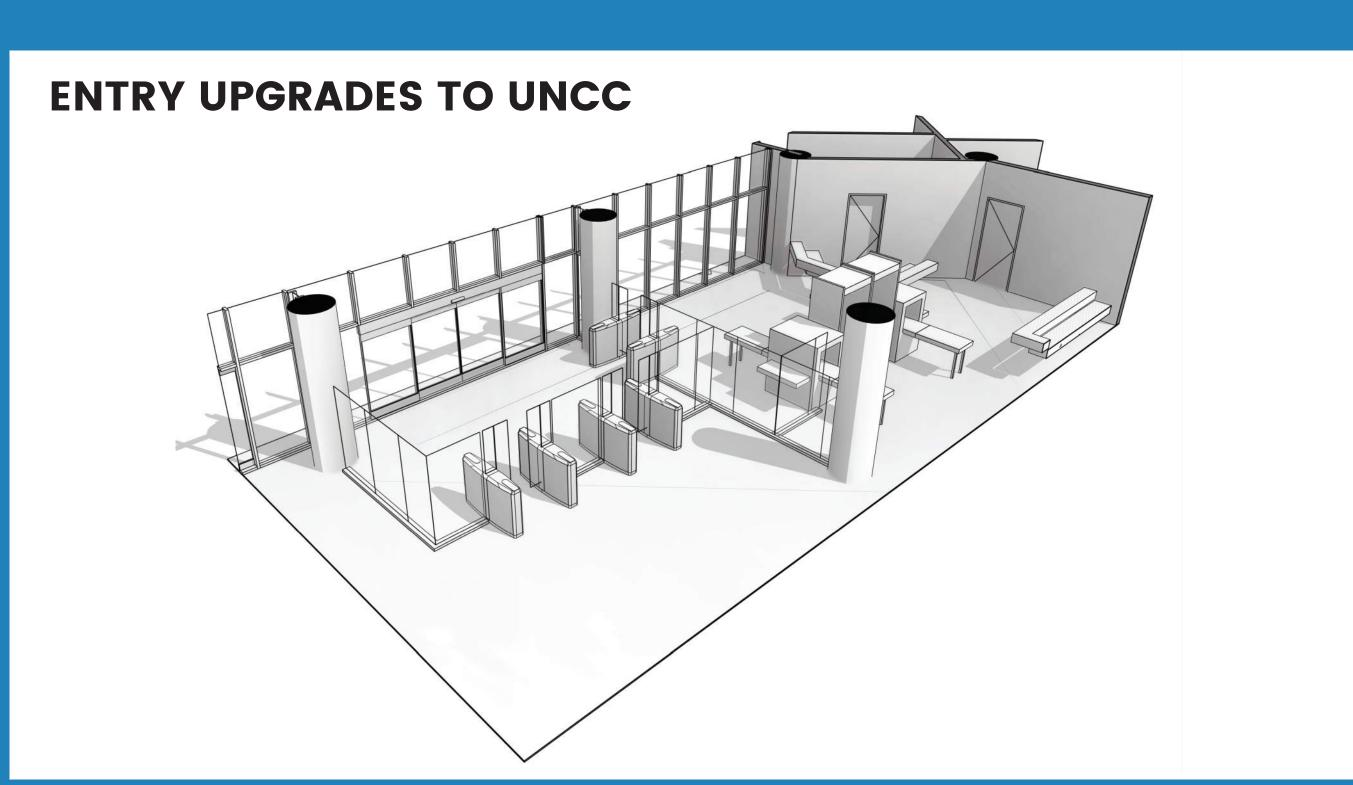
A proposed project is to upgrade the main entry doors to the UNCC building to enhance security and accessibility to the building. This will include motion activated doors and new Access Control systems where appropriate.
