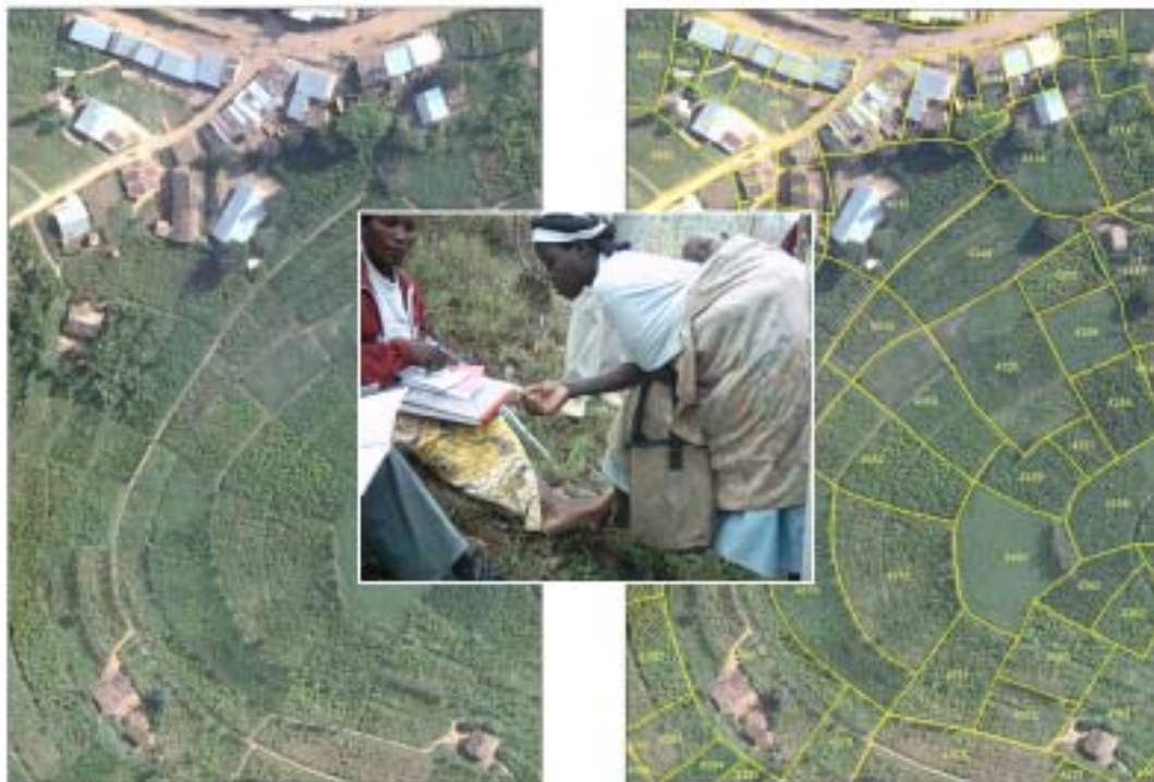
Figure 4. Example from Rwanda showing aerial imagery (left), from which the parcel boundaries are easily identified (right). This is essentially a participatory approach undertaken by locally trained land officers Source: Didier Sagashya, Rwanda
