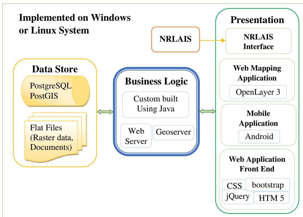
Figure 1: Overview of AIIMS-CCF System Architecture
